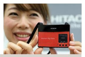
The badge: measuring motion, interaction, movement and voice. A credit card-size wearable device loaded with sensors that determine where the wearer is, and whether he or she is sitting, standing, typing or nodding, talking (to whom) and for how long. The device is an enabler of people analytics, a data-driven approach to managing people at work, based on deep analysis of data.
