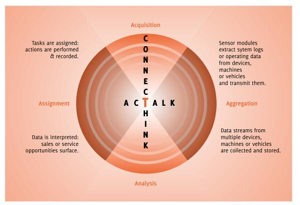
The architecture of any Internet of Things or Industrial Internet application consists of a four-tier structure in which the <u>Connect</u> phase is the start of data <u>Acquisition</u>; the automated communication phase (<u>Talk</u>) corresponds with <u>Aggregation</u> of data; <u>Think</u> equals data <u>Analysis</u>; and <u>Action</u> follows upon the (automated) <u>Assignment</u> of tasks.
