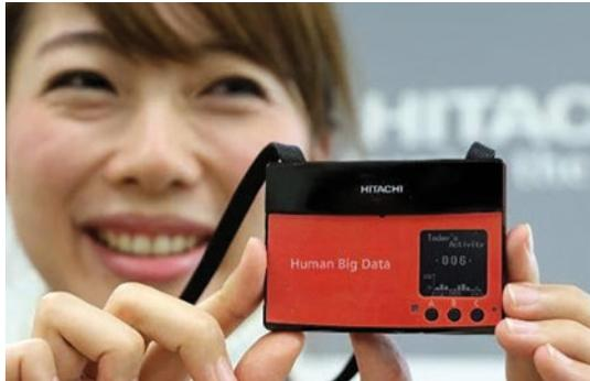
The badge: measuring motion, interaction, movement and voice. A credit card-size wearable device loaded with sensors that determine where the wearer is, and whether he or she is sitting, standing, typing or nodding, talking (to whom) and for how long. The device is an enabler of people analytics, a data-driven approach to managing people at work, based on deep analysis of data.
